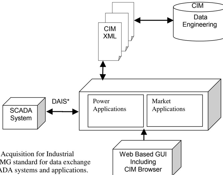
\*DAIS: Data Acquisition for Industrial Systems = OMG standard for data exchange between SCADA systems and applications.
